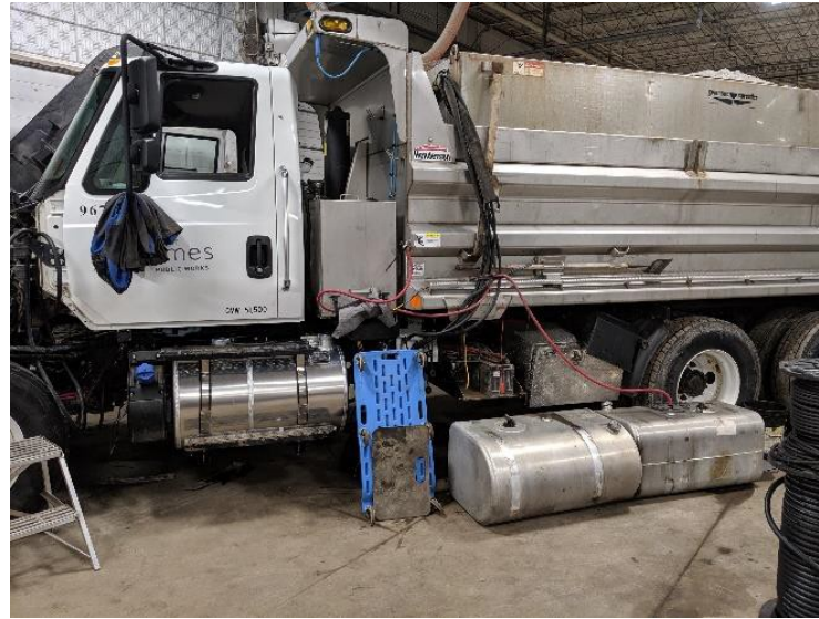
Truck #967 in January 2020 with new split tank and Optimus Vector being installed
